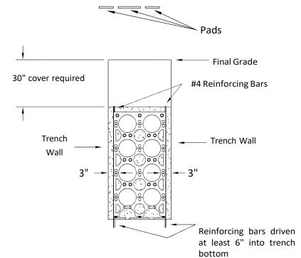
(F) To properly support multiple ducts in a trench, the duct spacers are separated approximately 6-1/2' to 7' apart. Contractor is required to use 20' lengths, this means there are three (3) spacers installed within one section of duct.
