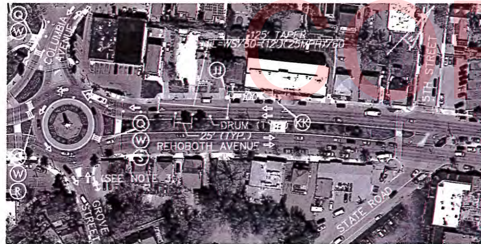
PHASE 3 TRAFFIC CONTROL DETAIL
